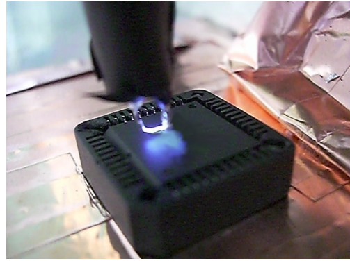
Figure 2. Spark-gap burst right above the surface of a microcontroller
