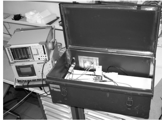
Figure 3. Shielded box with utilized spectrum analyzer and DEMA/DPA measurement setup.
