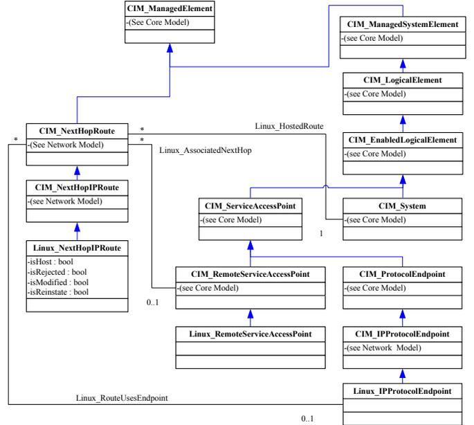
Fig. 3. Cut-out of the network CIM-schema constitution
