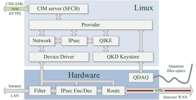
Fig. 2. System-on-chip architecture of our prototyping platform
